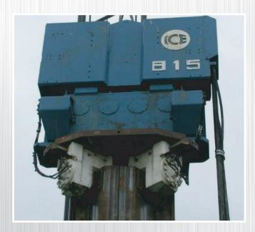
The single clamp vibro is replaced with a Double Clamp assembly. In Europe double clamps are used extensively and now slowly being adopted in the US.
